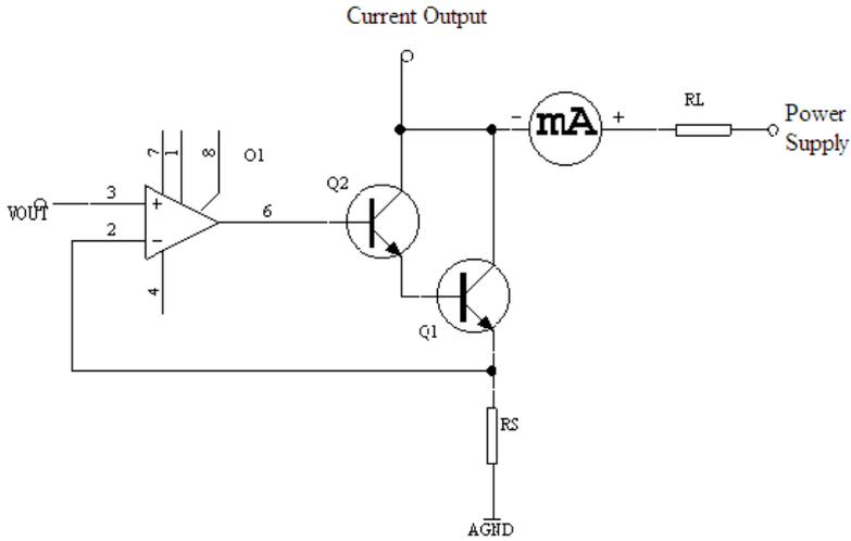
External power supply:  $V_{pwr}$ ;  $V_{pwr}$  range:  $R_L \cdot I_{Out\_max} + 7V \leq V_{pwr} \leq 36V$ , connect the external power supply ground to the board's ground.  $I_{Out\_max} = 20mA$  when the output range is 4~20mA,  $I_{Out\_max} = 10mA$  when the output range is 0~10mA.
